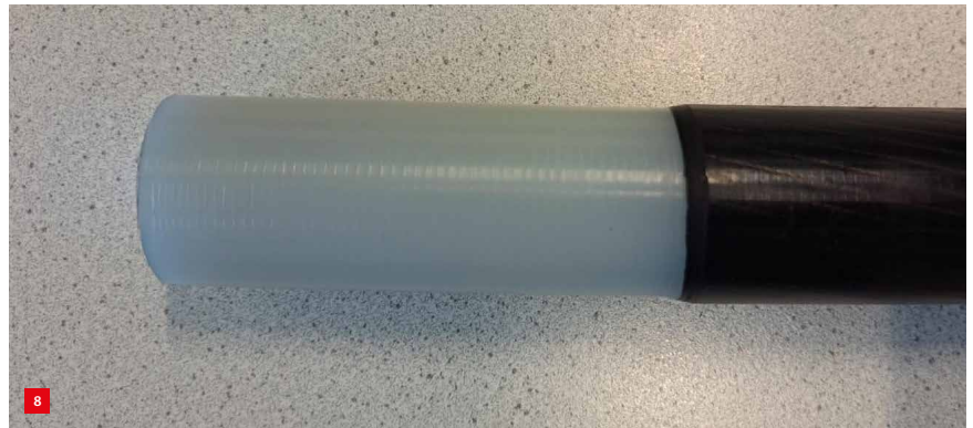
Result of the drive system test. The insulation will be partly removed at a later stage.
